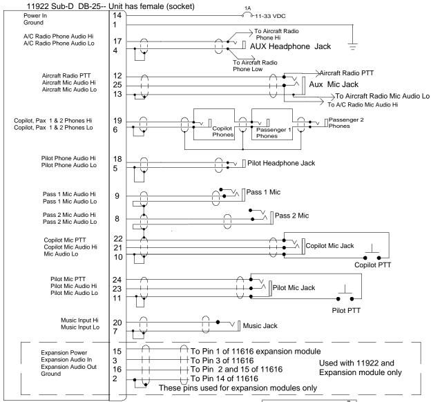
All wire must conform to MIL-22759 or 27500. Minumum 24 gage shielded wire.
